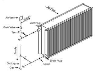
Figure 7: Vertical Air Flow
