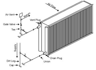
Figure 5: Vertical Air Flow
